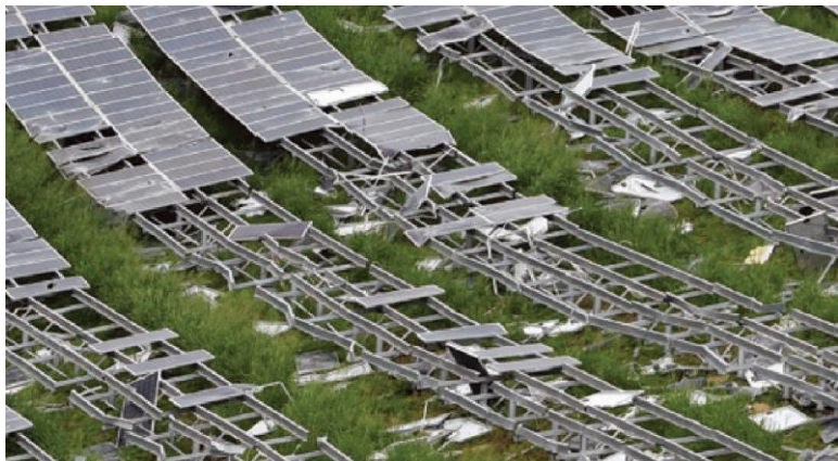
"Zipper" failure of PV modules using common midclamps
